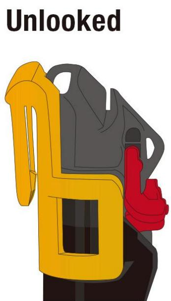
① Lift the red blade cover upward.
