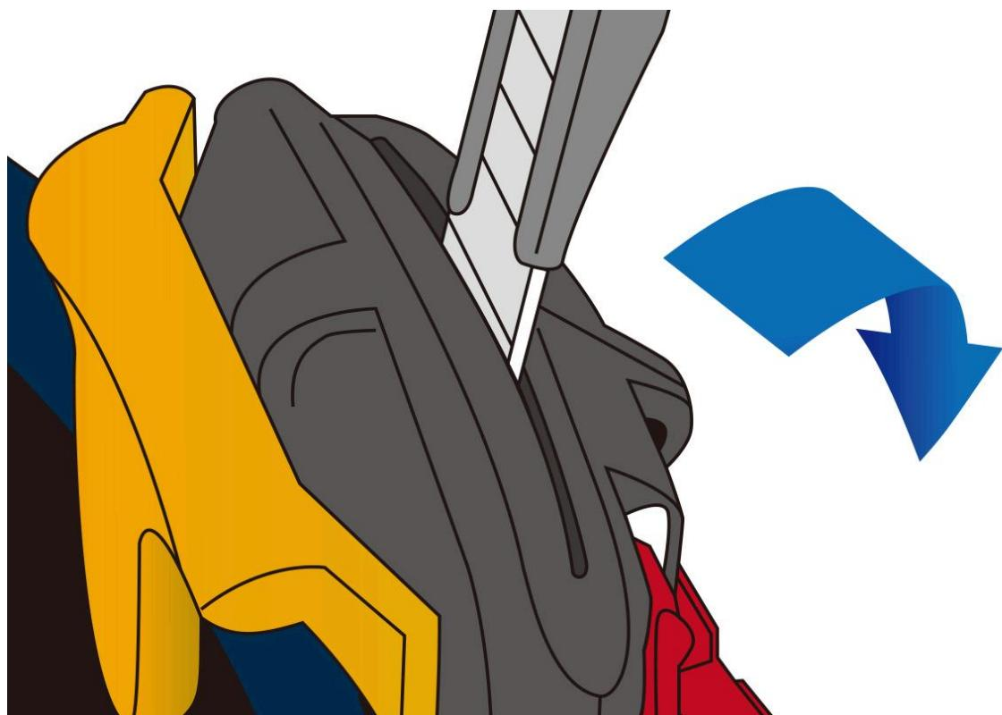
① Insert the blade into the blade snapping slit with exposing one blade segment only.
